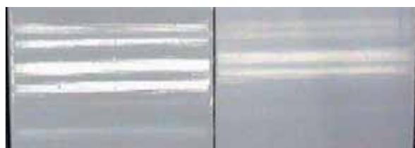
0.06% K-KAT XK-614 paint aged 4 hours before application vs. 0.04% DBTDL paint aged 2 hours before application
