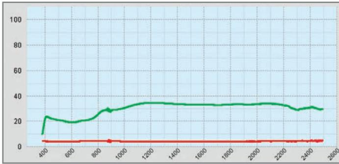
**Fig. 6 Reflectance curve for IR reflecting black oxide (in black, average TSR of 30%) and traditional black oxide (in red, average TSR, 5%)**
