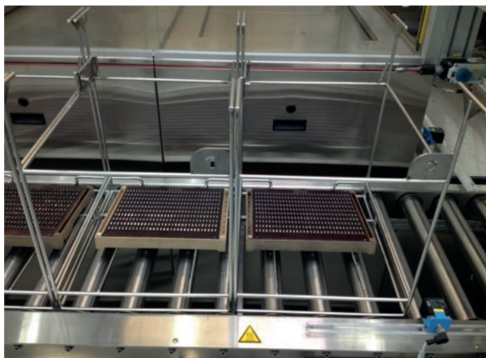
Indexable inserts and boring tools are cleaned in carriers immediately prior to coating
