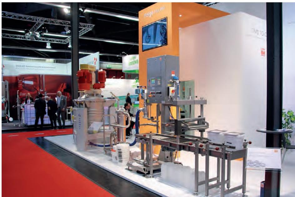
As an option, lid roller type RBB-Dn with integrated lid control station perfectly rounds off the process. The lid roller reliably closes and then checks the lid that is placed onto the pail.
