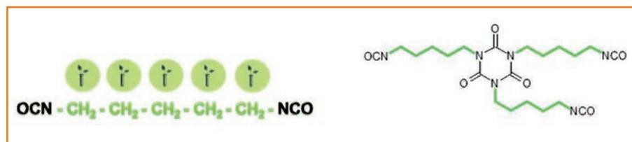
**Fig. 3 Structural formulas of Pentamethylene diisocyanate (PDI) and PDI trimer. The carbon atoms from biomass are shown in green**
