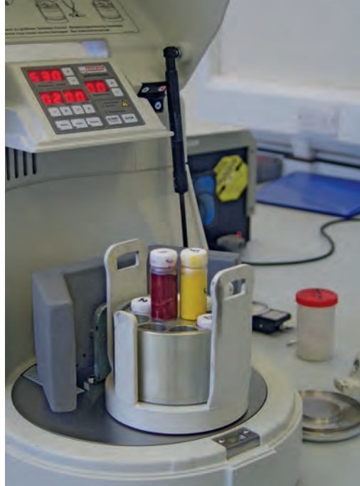
Fig. 2 Bead milling and dispersion system for laboratory experimentation that can grind or disperse powders in suspension
