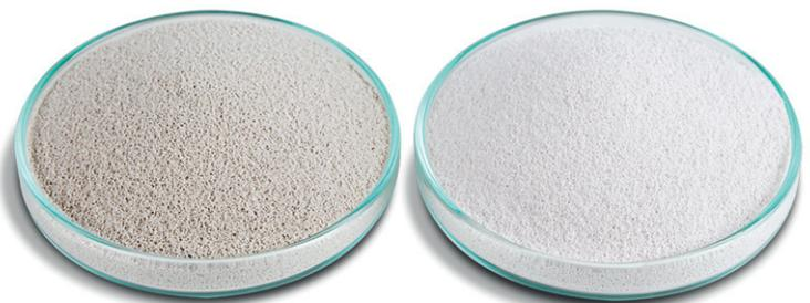
**Fig. 6** Colour comparison of Poraver (on left) and Poraver X granules
