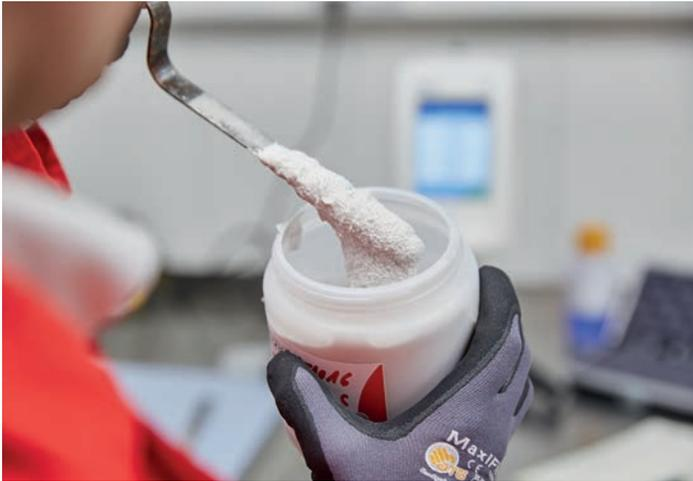
**Fig. 2** Sample of ready to use base coat mortar with Poraver X
