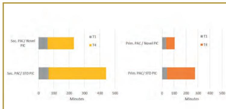
**Fig. 1** Drying time comparison at room temperature (23°C, 50% RH) of different WB 2K coatings (based on secondary and primary acrylic polyol and two different hardeners) according to DIN 53150, 120 g/m<sup>2</sup> on glass. Total dry (T4) of WB 2K systems can be reduced by half compared to a standard system when using the novel hardener
