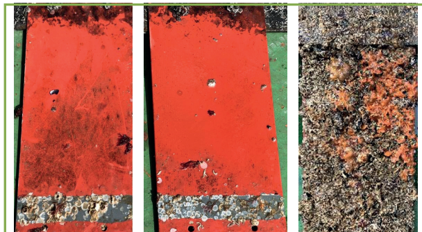
Fig. 1 Standard 32% \text{Cu}_2\text{O} . Fig. 1B VP 4200 : \text{Cu}_2\text{O} 4% :12%. Fig. 1C Blank (PVC Reference) 32% standard \text{Cu}_2\text{O} . Fig. 1B VP 4200: \text{Cu}_2\text{O} 4%; 12%. Fig. 1C campione bianco (riferimento PVC)
