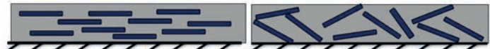
Fig. 5 Shows that the alignment of the barrier pigments is highly dependent on the remaining composition of the coating. A good alignment can only be achieved if the entire formulation is optimised to provide good barrier properties
