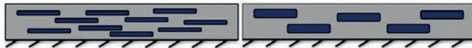
Fig. 4 shows that the barrier effect is highly dependent on the shape and size of the barrier pigment. Both images in the illustration show the same weight % of the barrier pigment
