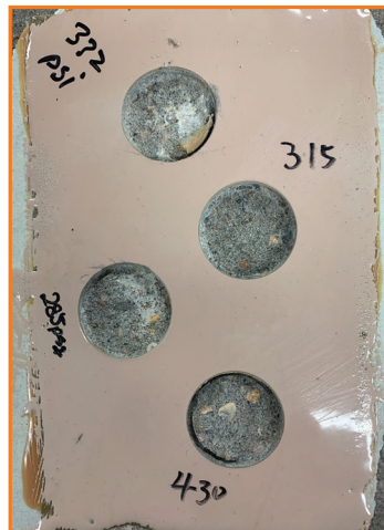
Fig. 2B 2K STPE/Epoxy Adhesion Strength Testing Results
