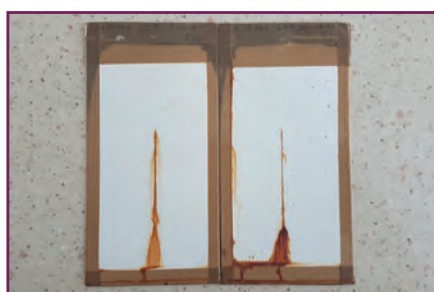
Fig. 1 Corrosion resistance after 72 and 240 hours
