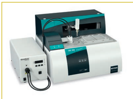
Fig. 1 Photo-DSC 204 F1 Phoenix® with OmniCure® S2000 lamp for UV curing Photo-DSC 204 F1 Phoenix® e lampada OmniCure® S2000 per la reticolazione a UV
