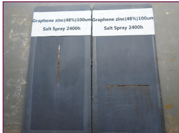
Fig. 3 Graphene used in a 2K water-based epoxy system having 48% of dry substance of zinc (D50: 13 \mu\text{m} ) and 1 % dry substance of Graphene
