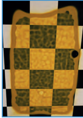
Fig. 2A Pigmented Acrylic-based clear coating without substrate wetting additive Vernice trasparente acrilica pigmentata senza additivo bagnante
