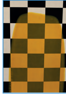
Fig. 2B Pigmented Acrylic-based clear coating, within 1% of substrate wetting additive Siltop 715 Vernice trasparente acrilica pigmentata con l'1% di additivo bagnante Siltop 715
