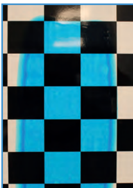
Fig. 4A Pigmented Polyurethane-based clear coating, without surface levelling additive Coating trasparente pigmentato a base PU, senza additivo livellante
