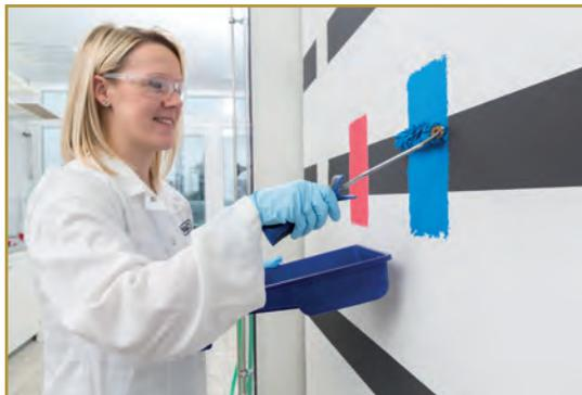
**Fig. 3 A lab assistant checks the hiding power of paint**
