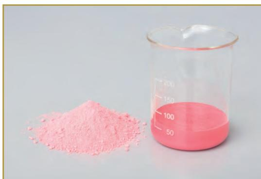
**Fig. 1** Paint containing NEXIVA® in powder form (left) and redispersed with water (right)
