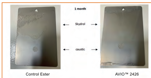
Fig. 4 Chemical resistance test results for 2K PU coatings formulated with Avio™ 2426 (right) confirm enhanced performance relative to a commercial polyester diol (left) alternative for caustic and Skydrol
