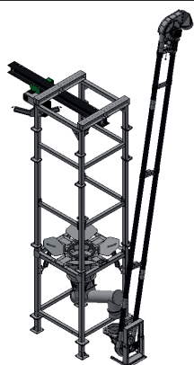
Svuota big bag + aeromeccanico Big bag discharger + aeromechanical conveyor
