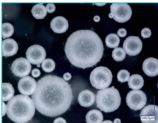
Under the microscope, the shape of Poraspheres is recognizable as a hollow glass sphere (Picture PORAVER)
