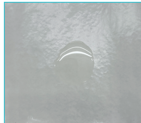
Appearance after dripping vegetable oil onto a coated surface and leaving it for 24 hours
