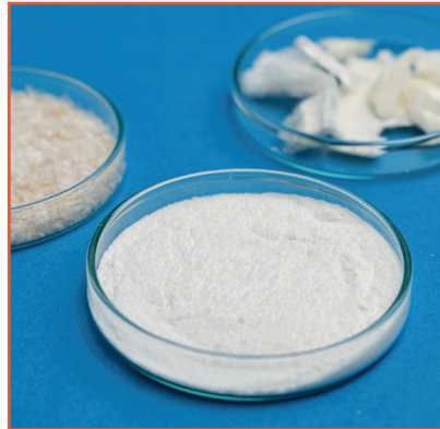
Fig. 2 - To produce high-purity chitosan from insect exoskeletons, chitin is isolated, purified and converted
